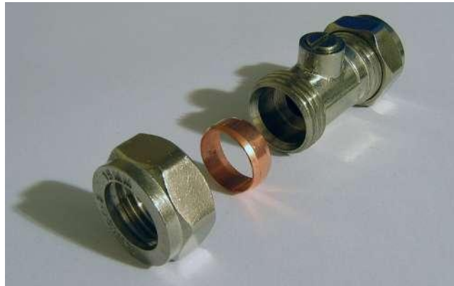
Above: a compression-fitting isolation valve, 15mm pipe diameter, screwdriver-turn
