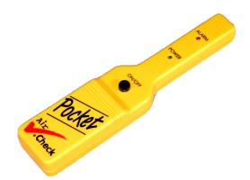
The Pocket Air Check® measures 6-1/4" x 1-3/8" x 3/4" and weighs approximately 3 ounces. Its highly sensitive solid-state sensor detects natural gas, propane, hydrogen, butane and more, locating leaks in pipes, valves, fittings and tanks. The instrument provides both audible and visual alarms, and operates up to 8 hours on 2 AA batteries.
